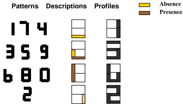
Figure 0.12. Confusion patterns for numerals visualized from the patterns’ data analysis descriptions in terms of edges being present or not. The right-hand part presents profiles of the common edges, for comparison.
