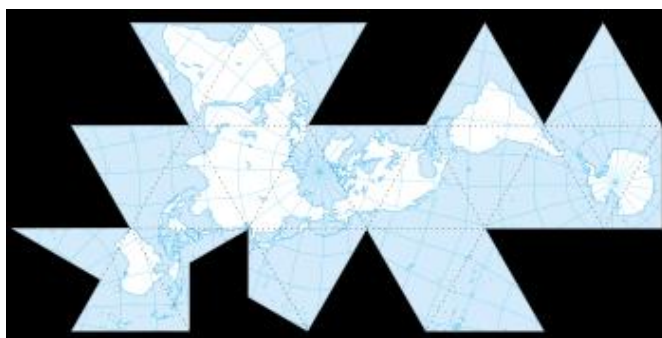
Figure 0.4. The Fuller Projection, or Dymaxion Map, displays spherical data on a flat surface of a polyhedron using a low-distortion transformation. Landmasses are presented with no interruption.
