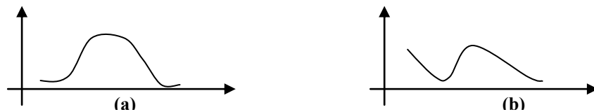
Figure 4.3. One-modal distribution shape on (a) versus a two-modal distribution shape on (b): the standard deviation of the latter is greater, thus making it less significant under the z-scoring standardization.
