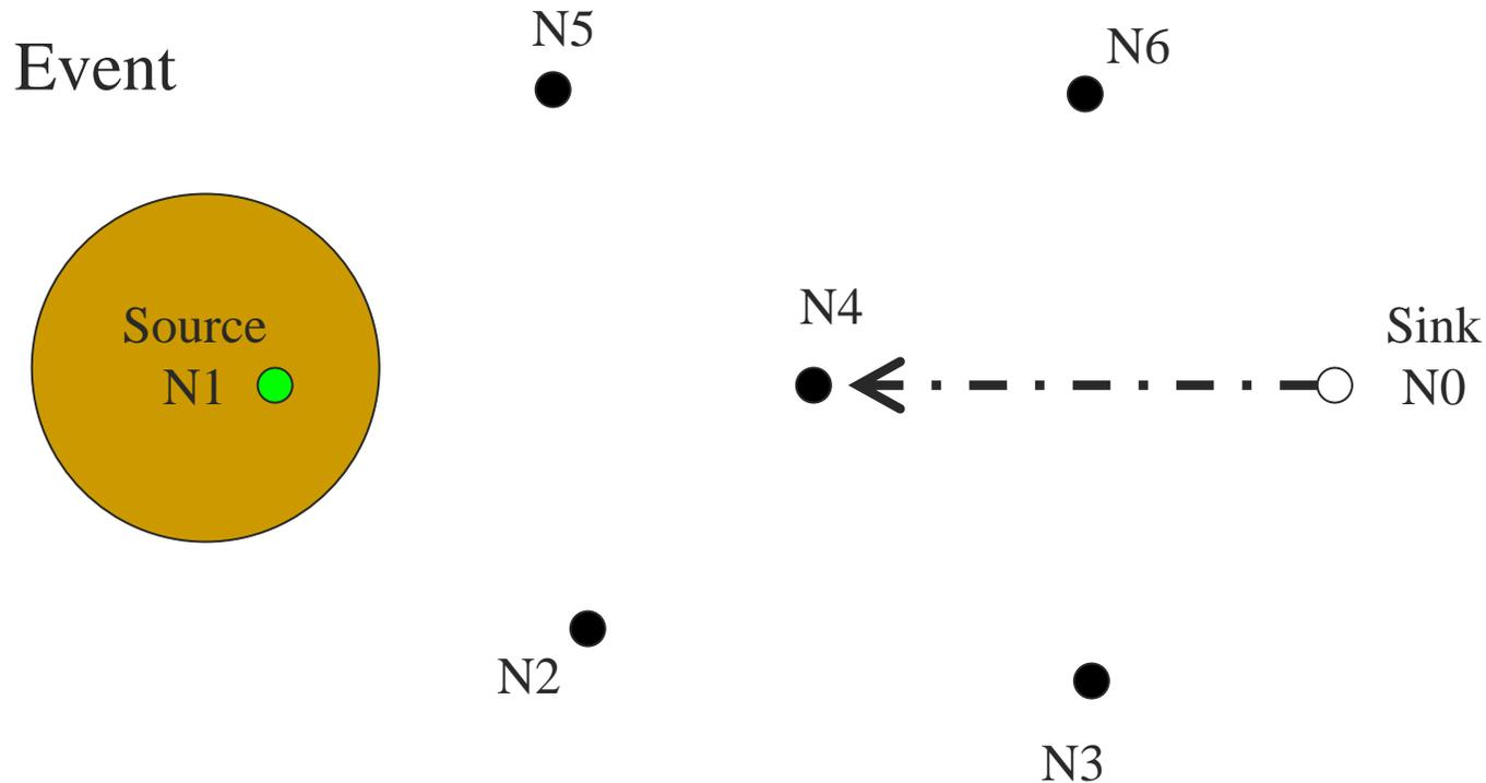
The sink **reinforces min-delay path**, by sending the same interest to neighbor N4 with higher requested data rate.
