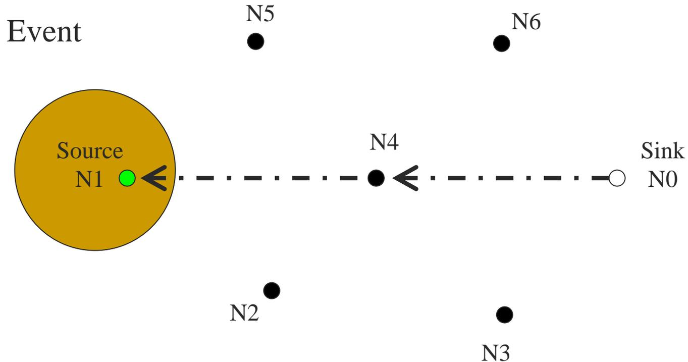
N4 reinforces min-delay path, by sending the same interest to N1 with higher requested data rate.
