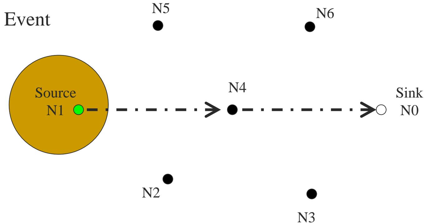
The source propagates event records to the sink along the reinforced path with a high frequency.
