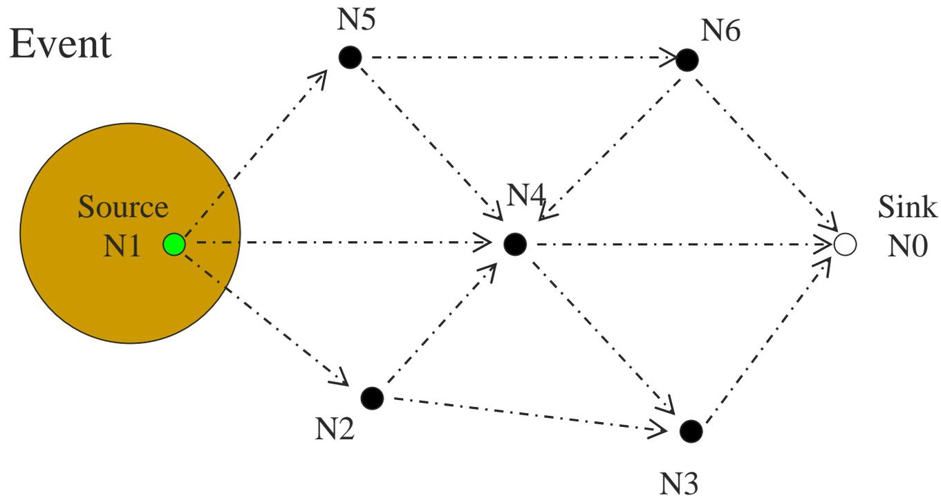
Event records are propagated back to the sink through **multiple paths** at the initially **low data rate**.
