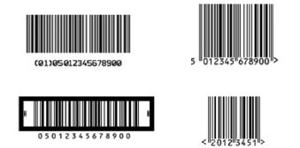
Fig. 2.3. Clockwise from the top left: samples of UCC/EAN-128, EAN-13, EAN-8, ITF 14.
