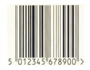
Fig. 2.1. A typical example of an EAN-13 bar code.
