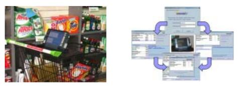
Figure 1: Prototype shopping cart implementation: Shopping cart with tablet PC, wireless network and RFID reader (left). User Interface: Login screen, shopping options including shopping cart content monitor, shopping list, total shopping cart content cost, offers and personalized promotions, additional product information and finally, fast check-out (right).
