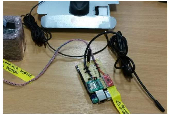
Figure 4: Deployable device hardware. From left to right: Battery, IoT platform with added SD card and accelerometer, and thermal probe.
