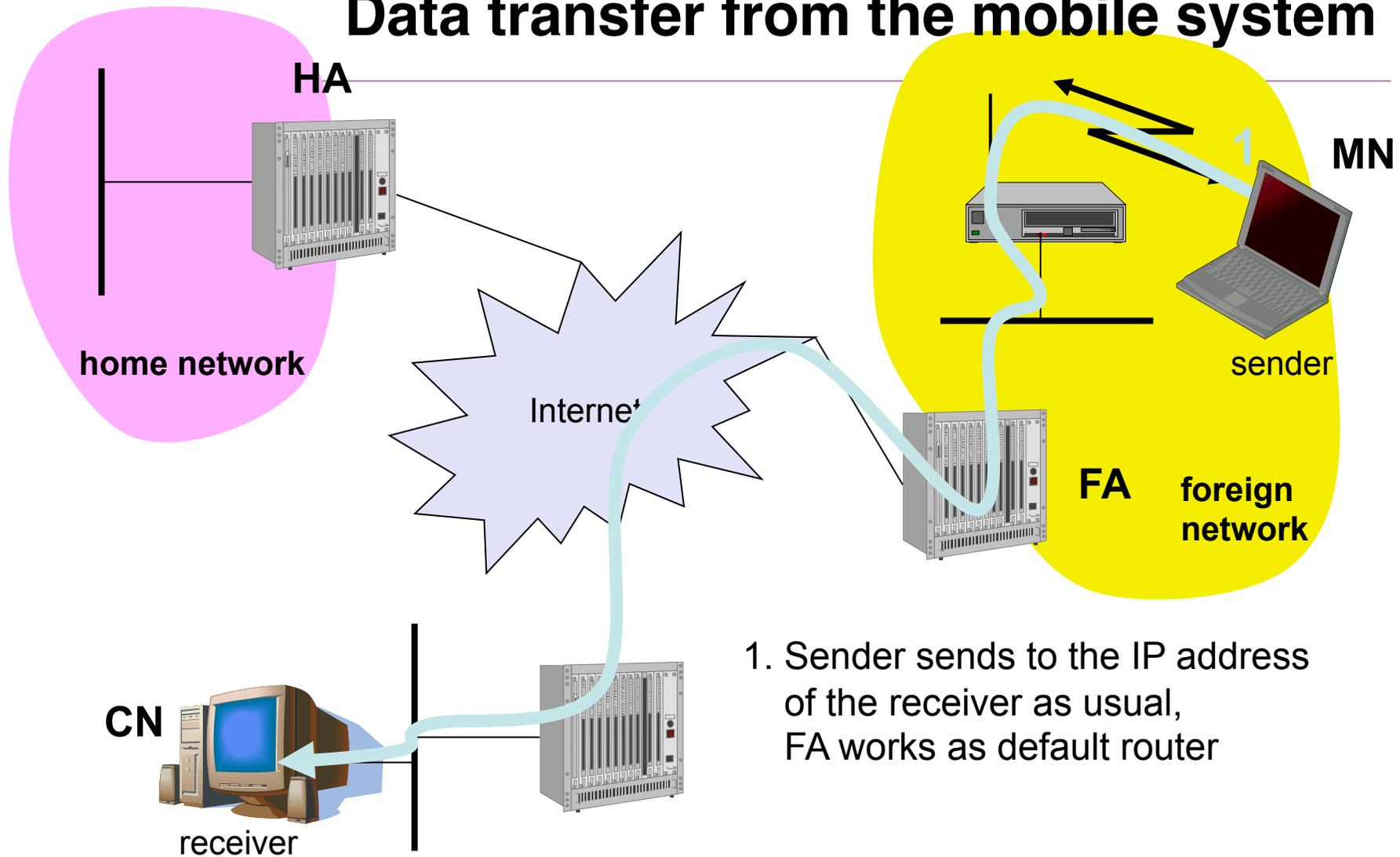
1. Sender sends to the IP address of the receiver as usual, FA works as default router
