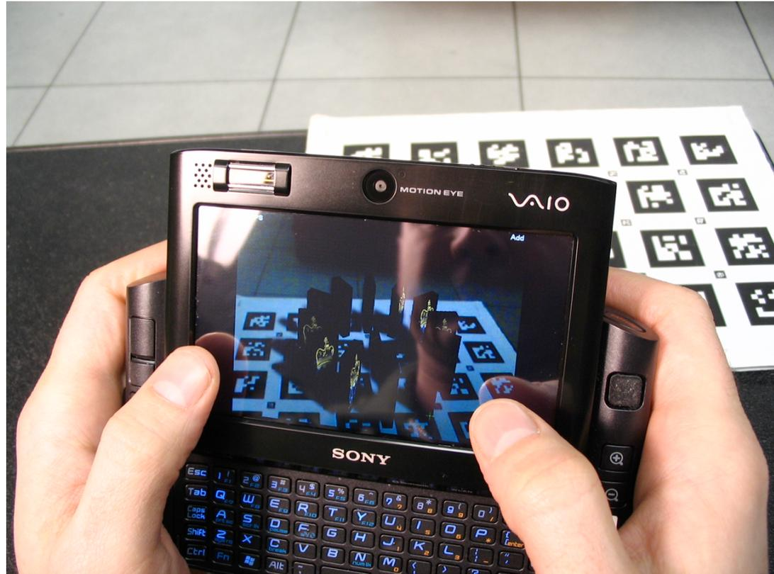
Using fiducials to overlay information e.g. 3D object models, on images captured via the mobile phone camera. Fiducials are used to provide the location where information will be superimposed.
