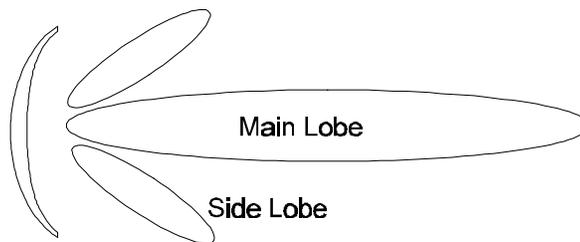
***Figure 5: Radiation Pattern of Directional Antenna***
