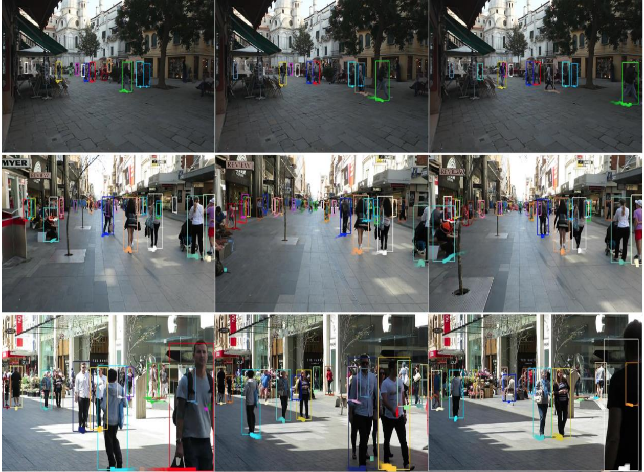
Fig. 12. Some qualitative results on the MOT16 benchmark: the same identity labeled by box with the same color.
