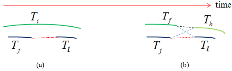
Fig. 2. High-level motion contexts: (a) Interaction between tracklet association (T_j, T_l) and tracklet T_i ; (b) Interaction between two tracklet associations (T_f, T_h) and (T_j, T_l) .
